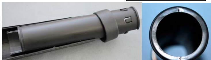
Preparing the focuser assembly. Note how the tongue and groove line up in the photo on the right.
