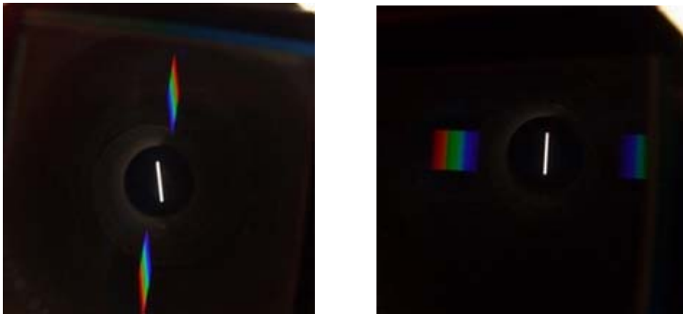
Fig.7: Incorrect and correct setting of diffraction grid with respect to the slit
