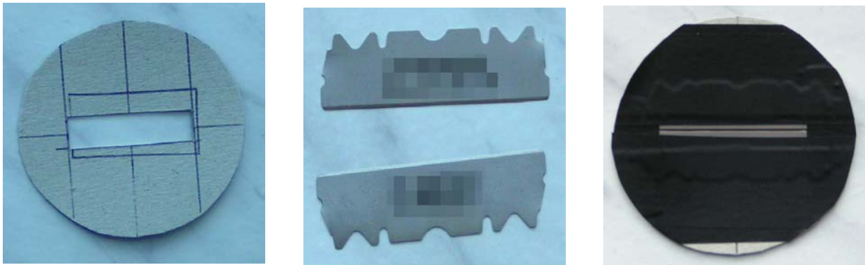
Fig. 5: Elements of slit and ready-made razor blade slit
