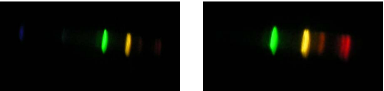
Fig. 15: Spectrum of a street mercury-vapour lamp
