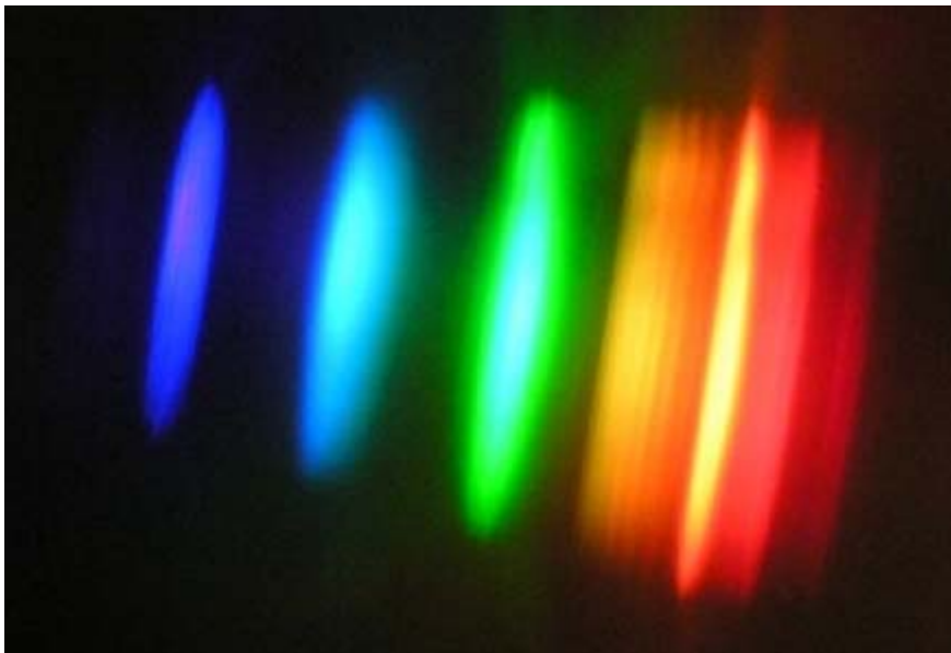
Fig. 11: Spectrum of an energy-saving bulb
