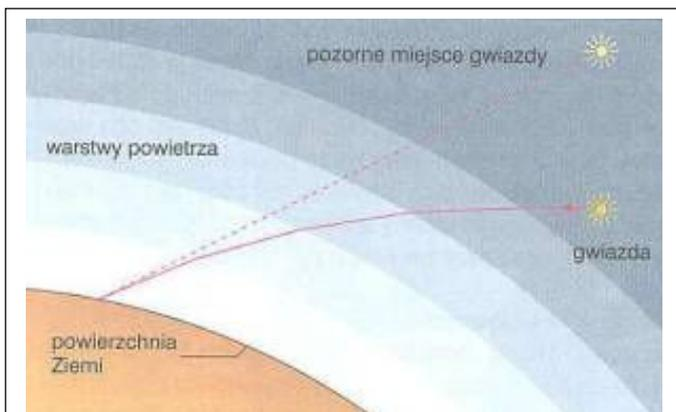
Fig. 4. The trajectory of light rays – phenomenon of refraction.
