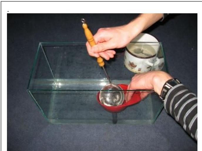
Fig. 2. Pouring a brine to the bottom of the aquarium is a key stage in the experiment.
