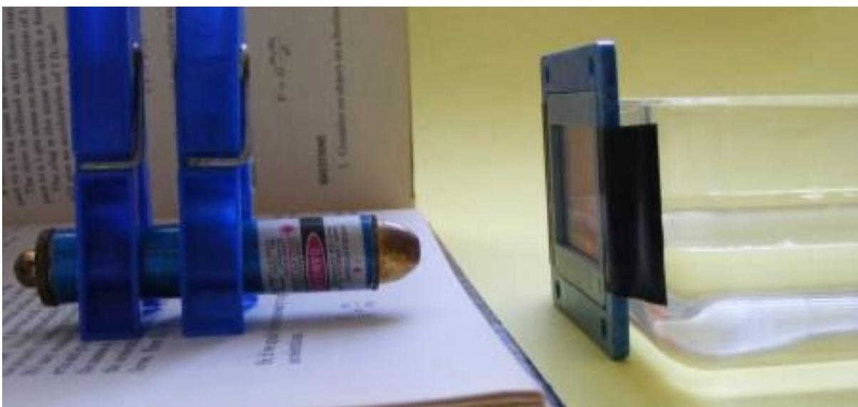
Fig. 4. Placement of laser in relation to a vessel with liquid
